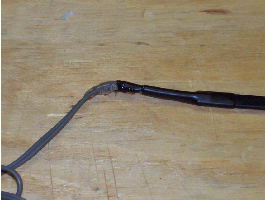
Seal the end of the temperature probe with glue.
