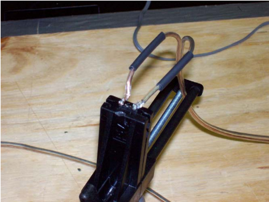
Solder both wires to the plug terminals.
