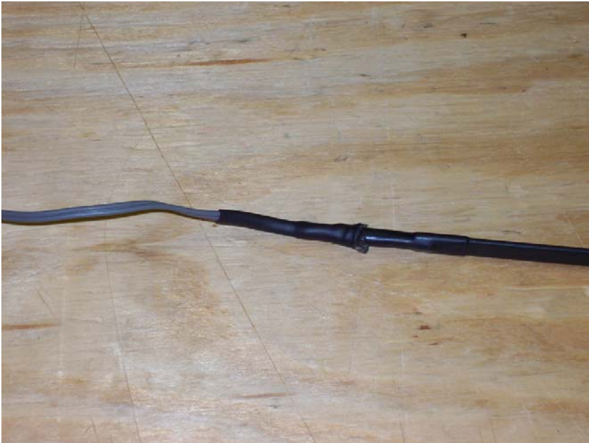
Cover the end of the probe with heat shrink tubing.
