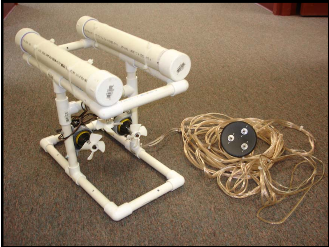
Figure 1.1: An ROV built from PVC & Bilge Pump Cartridges. The design can change depending on the builder's desires and the robot's underwater objective.
