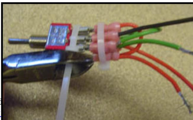
8. While holding the controller the easiest way to “steer” it corresponds with how the ROV moves through the water. After launching the ROV, if pushing the L and R switch forward, the ROV goes forward, you’re in good shape. **If pushing the switch forward causes the ROV to reverse the solution is easy.** Just take the wires connected to the power source and switch them, i.e. switch the polarity. The ROV will now move forward when the horizontal thruster switches are pushed forward.
