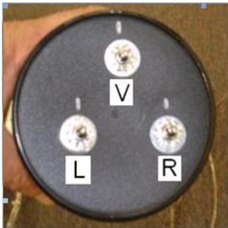
4. **Before you launch the ROV use your allen wrenches and soft pliers to make sure that the props and prop adapters are snug on the bilge cartridge hub.** If they spin off on the test put 'em back on. Check the propeller hub nut and also the smaller set screw that keeps the propeller attached to the hub. The smaller set screw is small and somewhat delicate. Don't over tighten these, they'll break.
