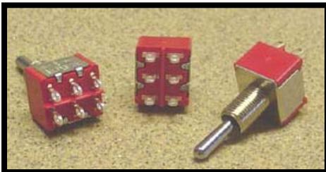
Figure 6.1 shows three views of the same switch. Note the six posts of the switch back in the left and center view. Each of the six posts will receive a specific wire. The right-most view shows the toggle that actuates the switch when it is pushed up or down.
