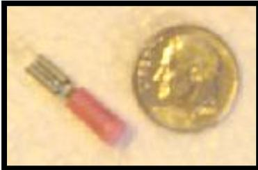
Get six (6) female quick disconnect vinyl insulated connectors ready to attach to the wire ends (Figure 6.10 and 6.10b). These connectors should be able to accept 18-22 gauge wire. The idea here is that the female end of the connectors fit snugly onto the switch posts..
