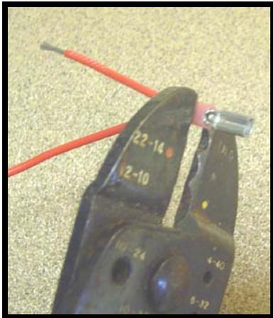
Slip the connected end into a connector and crimp it (Figure 6.19). This will bind the two wires securely. Attach another connector to one of the other bare wire ends. Don't worry about the other bare end. It will be connected to the tether wire. Do the same for the green wire. Now we should have the four sets of wires as pictured in Figure 6.17.
