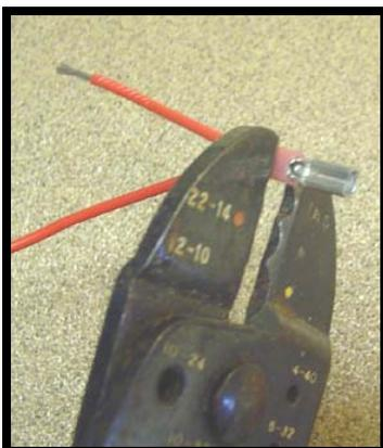
**Figure 6.12:** Hold the insulated part of the wire connector in the jaws of the crimping tool. Squeeze the insulation until the insulation is pinched. Do not apply too much pressure or the connector will break.
