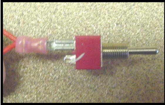
After the connector has been adjusted with the gentle squeeze, it should require a small amount of force to slide it over the post (Figure 6.16).
