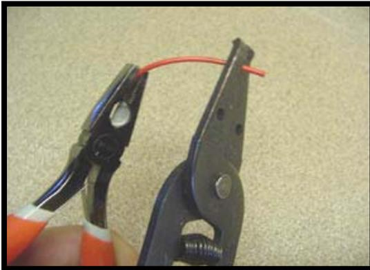
About 3/8" of an inch of insulation needs to be stripped from one end of the wire and 1/2" from the other end. Because of the small size of the wire pieces this can be a little tricky. Grasp a wire piece with the flat jaw pliers (2) with one hand and place the jaws of the wire stripper (4) about 3/8" from the piece end. Squeeze the strippers and pull towards the wire end (Figure 6.7). The goal is to remove the insulation from the wire without cutting the wire strands (Figure 6.8).
