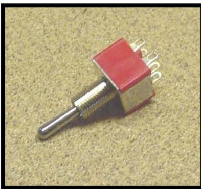
The gold colored annulus, or ring, around the silver switch is threaded so that you can fasten it to the handheld controller device (Figure 6.2). Each controller will have three of these switches, one for each thruster.
