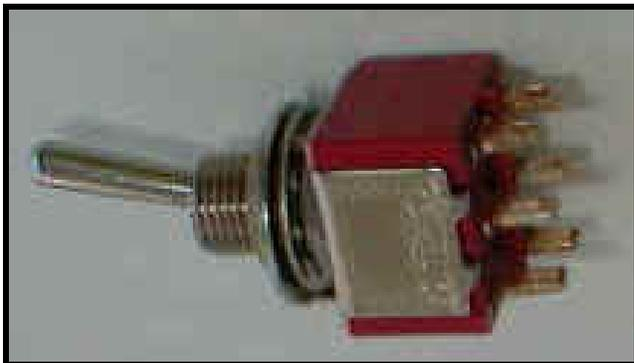
**Figure 6.15:** View of switch posts for connections.
