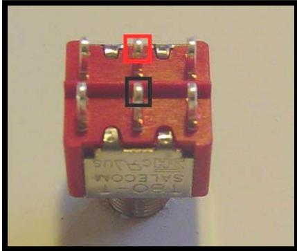
**Figure 6.21:** Attachment posts for the power wires which are red and black.
