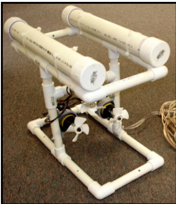
Figure 2.8 The PVC Pontoons are affixed to the ROV frame using Plastic Cable ties. The pontoons should not "wiggle". They should be firmly attached.
