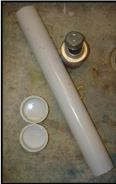
Figure 2.7: What you need to construct the pontoons. 1 15" section of 1.5" PVC, 2 end caps, and some stinky plastic cement.
