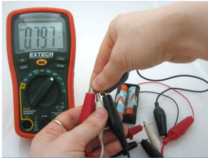
With my fingers on the sensor, heating it up a little, the temperature reading is now 29.7°C / 85.5°F
