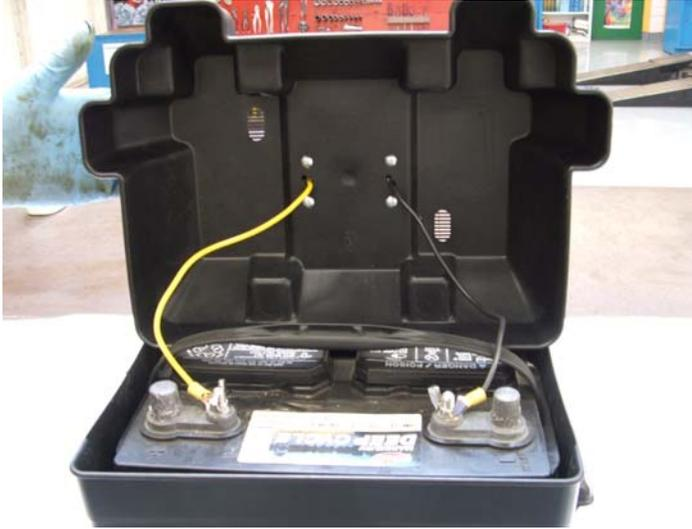
Close up of the connection between the circuit and the battery
